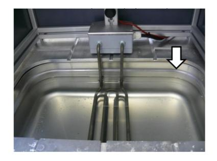
Close the door, plug in the power plug an turn on the device by using the main switch.Turn on the heating element by using the key switch below the display. Put the cover on the water tank to speed up the heating process.
