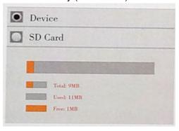
NOTE: If an SD card is inserted, SD card will be selected by default. Press the ENTER button to format the flash or SD card, press the F3 button to cancel the format, press Fl button to confirm the format.
