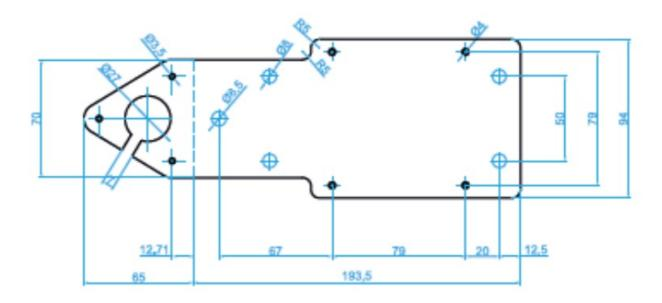
60-degree bending along dashed line, stainless steel, 2 mm thick
