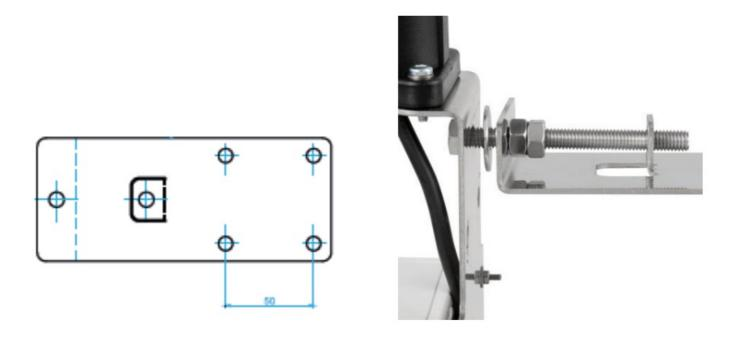
**ATTENTION:** When mounting the self-levelling additional bracket, make sure it is not completely tightened. It must be locked with the two M8 nuts in a way that it is still freely movable but without play! Observe the correct order of the connecting elements (see image).
