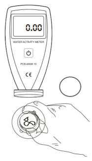
5. Start the instrument and combine the measuring chamber
