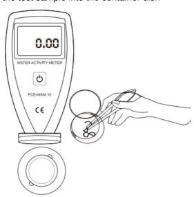
4. Put the container dish with sample into the bottom box of the measuring chamber (do not cover the container dish).
