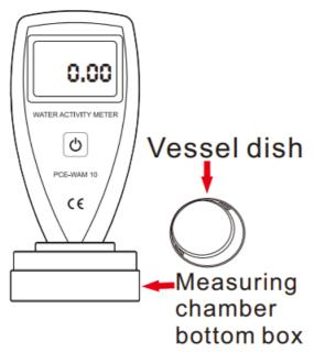
2. Open the instrument measuring room
