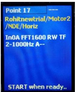
Attach sensor at the measurement point and press key.
