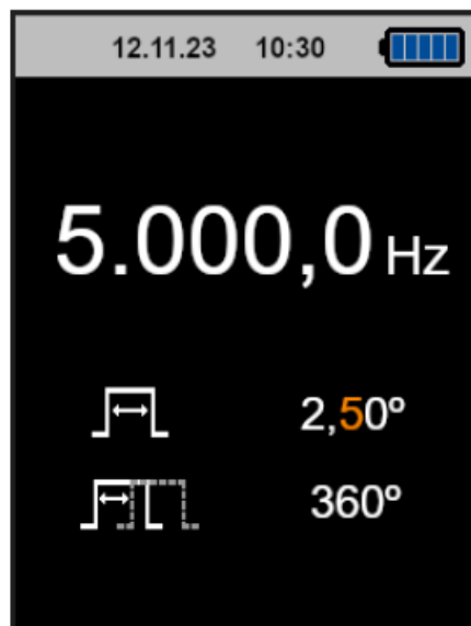
Figure 32. Quick mode - duty cycle modification
