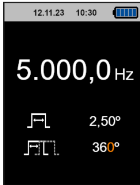
Figure 33. Quick mode - phase shift modification
