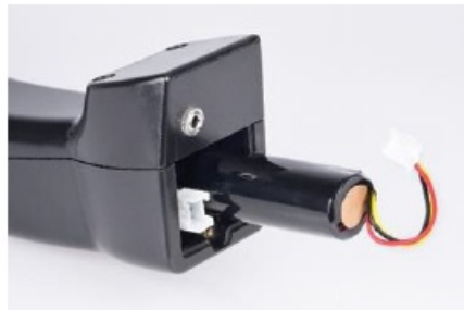
Carefully pull out the battery
