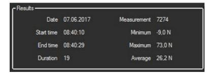
In this area, the following data are shown in numerical terms: start date of the measurement, start and end time, duration of the measurement in seconds, number of recorded readings, minimum and maximum value, average of all readings.
