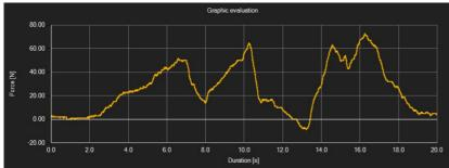
In the graphical evaluation area, the selected unit (force or pressure) is shown on the y axis and the time lapse is shown on the x axis. When moving the cursor over a dot on the displayed line, a small information box will appear
