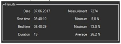
In this area, the following data are shown in numerical terms: start date of the measurement, start and end time, duration of the measurement in seconds, number of recorded readings, minimum and maximum value, average of all readings.
