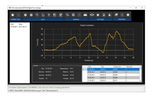
The main screen consists of several sections: Below the title bar, there is a tool bar with icons that can be selected by a mouse click. These icons are grouped according to their functions. Below this bar, you can find an area where the measuring points are displayed graphically ("Graphical evaluation"). To the left of the graphic, all series of measurements that can currently be loaded into the softwareare listed. The next section below the
