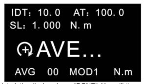
When the measurement is completed, the display shows "DONE". You will then see the average reading.
