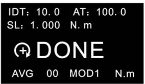
To reset the average value to start a new measurement, press the "Zero" key. The measured value is saved at the same time. Up to 10 average values can be saved.
