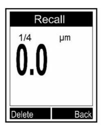
Press to enter the "Root" menu. Navigate to "Recall" with the very and confirm with. In the upper left part of the display, you will now see what value of a memory group has been selected (1/4). Select the desired reading with.
