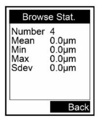
When making a measurement in measure mode, the current mean value, the maximum and the minimum values will be displayed below the current reading. To view the complete statistics, press first. In the menu that is now displayed, go to "Browse Stat." by using the keys and confirm with You can now see the statistical values of the currently selected memory group. To view the statistics of the other memory groups,
