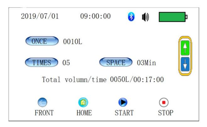
After setting the single sampling quantity, sampling times and sampling interval, press the START button to start program sampling. The grouping, location and delay of program sampling are saved by calling up the corresponding parameters of standard sampling directly. The total number of samples will be displayed in the data in the next row after setting the values of single sampling amount and sampling number.
