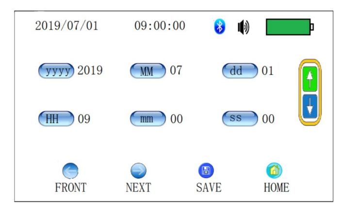
Press the key corresponding to year, month, day, hour, minute and second to select the corresponding parameter to be modified. When the parameter is selected, it can can be modified by using the up and down keys on the right.
