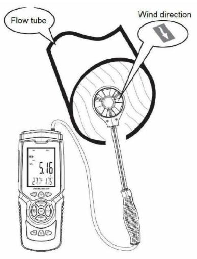
To make a measurement, align the flow sensor with the flow direction. An arrow inside the sensor indicates the orientation in relation to the wind flow. Wait for at least two seconds for the reading to stabilise.
