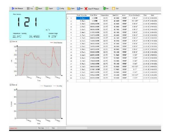
To set the read interval, click on "Option" and then select "Read interval(sec)". In the next window, you can set the interval in seconds.
