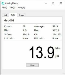
The "Group" tab displays all data saved on the meter. To export these data now, click on "Export". The data can now be saved to the PC as a CSV file. Click the "Sync" button to synchronise the software with the test instrument
