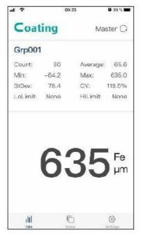
• Under the "Group" tab, the measurement data stored in the meter is displayed. Via the "Export" function, you can save the data on the mobile device as CSV, PDF and also as a TXT file
