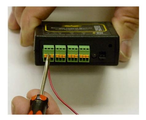
The LED for each Output will light when the Common Pin is connected to the Normally Open Pin. The LED will be off when the Common Pin is connected to the Normally Closed Pin. This is a latching relay, the relay state will not change when the power is removed form the ROM.
