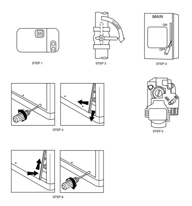
Fig. 6 – To Start Unit Electric Cooling
