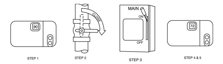
Fig. 7 – To Shut-off Unit Electric Cooling
