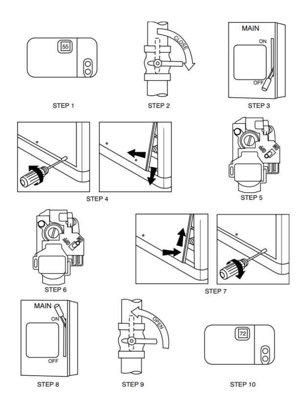
Fig. 5 – To Shut-off Unit Gas Heat
