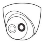
Turret (also known as `Eyeball') cameras contain their IR emitter separate from the camera lens, allowing them to be more powerful. Turret cameras resolve many pitfalls of the Dome camera, however at the cost of not being as vandal resistant and more obviously directional.
