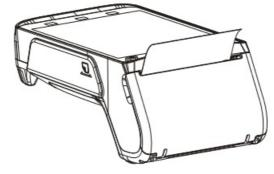
4. To tear the paper, press the paper downward along the cutter and pull it to the left or right along the cutting edge.
