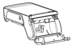
2. Insert paper roll with the end facing up and extending out of A930.
