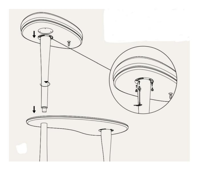
Apply the protective mats and tighten the screws
