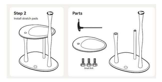
1. Align the holes at the bottom of the scratching board with the top of the wooden rod for installation
