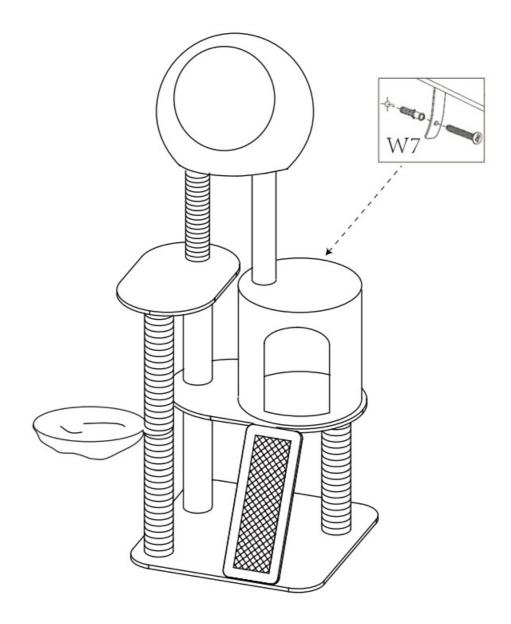
This is an antidumping belt that fixes the product to the wall and it can be used or not follow your needs. If it is a solid wall, please use expansion and self-tapping screws, if it is a wooden wall, only use self-tapping screws, please do not overtighten the screws.
