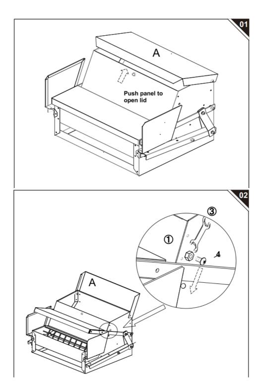
• **Tips**:To help chicken get used to the feeder, assemble part 4 screws and part 1 nuts in place, start assembling from the higher hole to lower hole, chicken will understand"step&open"rules of feeder finally.
