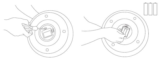
Unscrew the battery compartment cover with a screwdriver.
