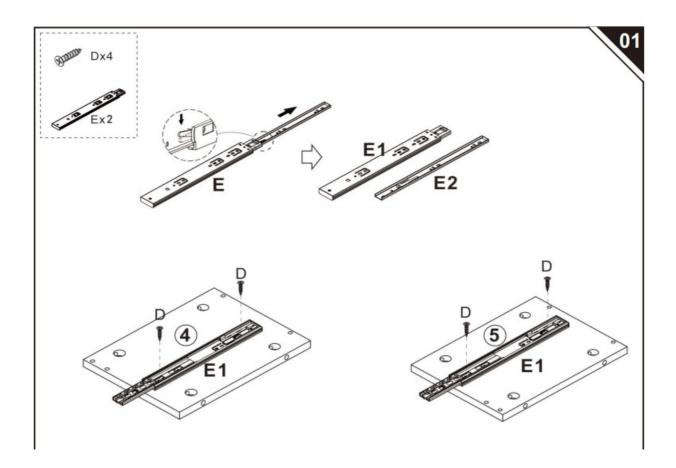
Please find the exact hole for installation, otherwise it will be misaligned. The screws on the drawer slide must be leveled, otherwise it will affect the smoothness of the drawer.
