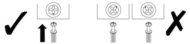
Quickfit head should be in the centre of the cam lock when the two panels are joined. Cam lock should be inserted before quickfit.
