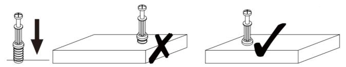
• CAM LOCK: When fitting cam lock, ensure starting position is correct before you insert connecting quickfit.
