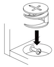
• Turn cam lock clockwise to tighten.
