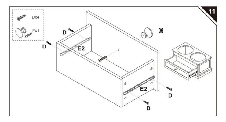
Be careful to push in the board when the both sides slide way been aligned.
