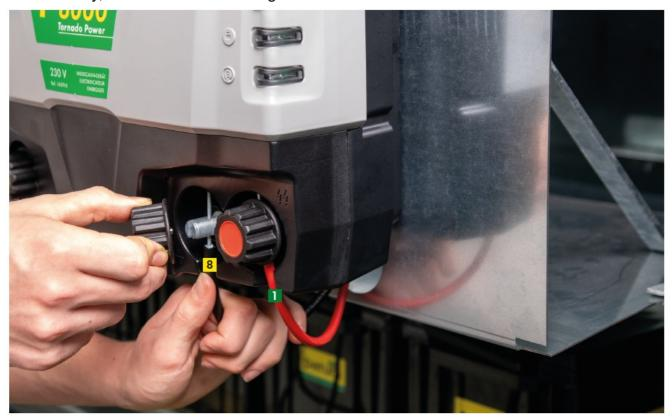
• **D:** When all cables are connected and all terminal screws are tight, the drawer can be pushed back into the box and secured with the screws.
