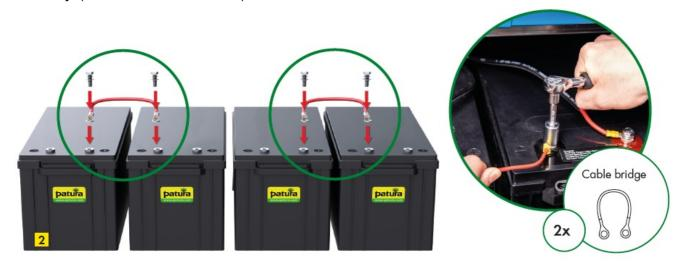
B: The two connecting cables of the batteries are already connected to the fuse holder and are now also attached to the batteries 2 using a ratchet and nut (size 13).
