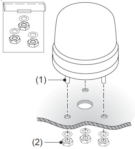
Insert the bolts of the beacon into the holes of the mounting surface. Use the nuts and washer (accessory) to secure in place.
