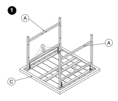
Please don't fasten the screw completely during assembly process. It will be likely to
