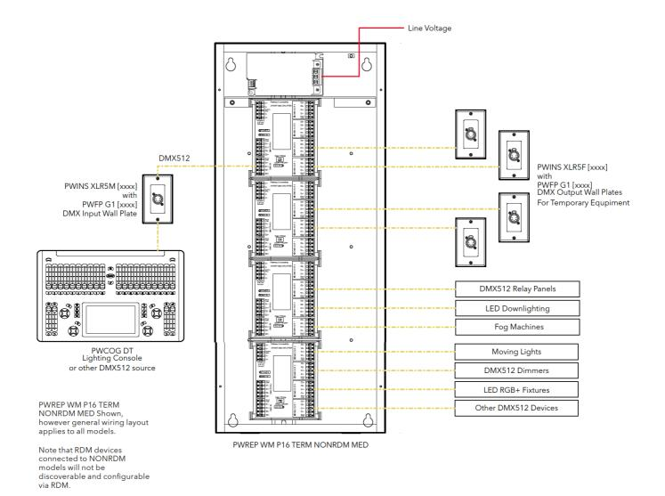
PWREP WM P16 TERM NONRDM MED Shown, however general wiring layout applies to all models. Note that RDM devices connected to NONRDM models will not be discoverable and configurable via RDM.
