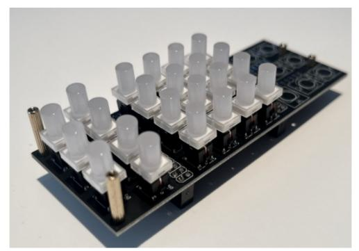
12. Carefully insert the mini jack PCB back into the control PCB. Screw both PCBs together using the metal spacers. Do not solder the pin headers at this stage
