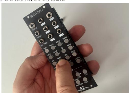
17. Carefully inspect the alignment of the buttons. From behind the PCB, look carefully for any empty holes with no pins inserted. Correcting soldering mistakes at this point will be extremely difficult. Once confirmed, proceed to solder.
