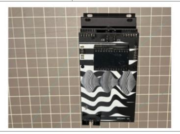
11. The trimmer on the right will calibrate CI and the trimmer on the left C9.
