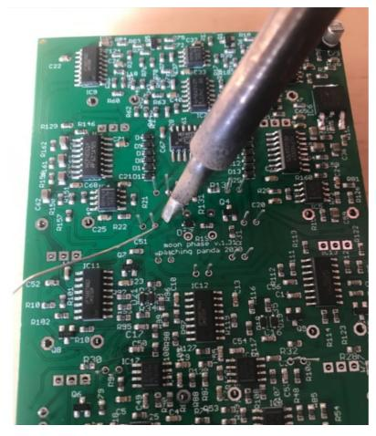
2. Put some paper tape, solder one leg and check if it's aligned to solder it. Continue with the rest of the soldering.
