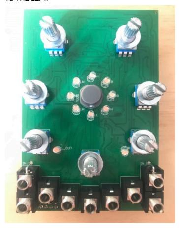
4. IMPORTANT BE CAREFUL WITH THE POLARITY OF THE LEDS. THE LONG LEG GOES TO THE POSITIVE.
