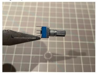
3. Place jacks, pots, 2 washers per pot and THE GRAY BUTTON MUST BE POSITIONED WITH THE FLAT SIDE TO THE LEFT.
