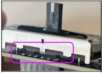
9. Position the button, ensuring the polarity is correct. Align the ! at the side of the button on the left with the on the side shown in the image.
