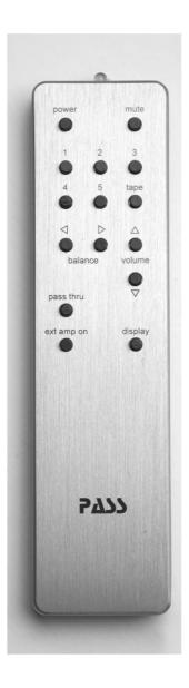
**Input Selection:** Pressing. 1,2,3,4,5 will immediately move the input selection to that input selection; volume and balance settings will not be disturbed.
