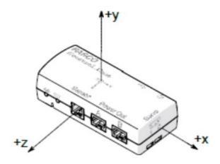
When motionless, the accelerometer measures +9.8 m/s2 when pointing away from the ground and -9.8 m/s2 when pointing towards the ground. This is useful for determining the //control.Node's orientation. For example, if the y-axis is pointing away from the ground, the Acceleration – y measurement reads 9.8 m/s2 and the other axes measure 0.
