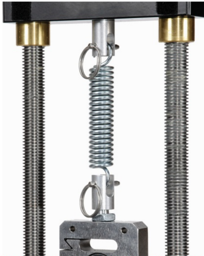
Figure 8. A spring secured in place using the Clevis Grip.
