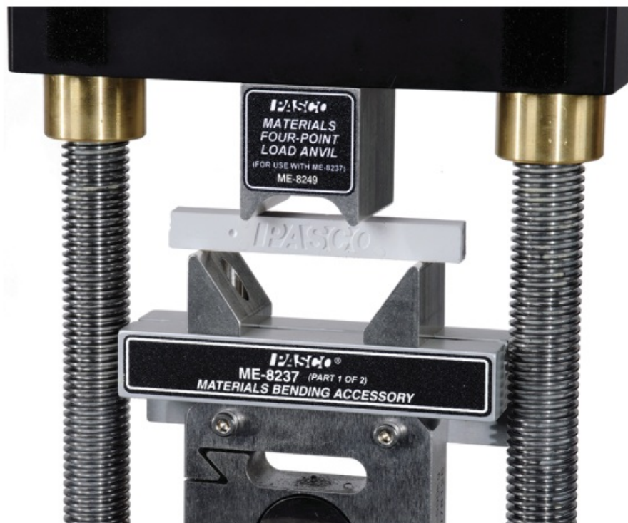
Figure 9. Testing a Cast Beam using the Bending Accessory and Four-Point Load Anvil.
