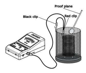
The proof plane is simply a small conductive disk mounted on an insulating handle. To sample the charge distribution on a charged object, simply touch the object with the proof plane, then place the proof plane inside the inner cylinder of the ice pail, *without* touching the cylinder. A charge of equal magnitude and sign is induced on the surface of the ice pail and can be read by the Basic Electrometer.
