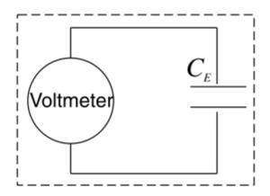
The capacitance of the electrometer alone is about 27 picofarads (pF). However, if the sampled object adds significant capacitance, the situation changes to what is shown in Figure 3, with *Cext* being the capacitance of the object. To accurately calculate the amount of
