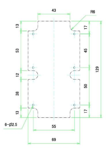
Note: The Tracker Carrier Board has a smaller bottom tab to provide space for the M8 connector.
