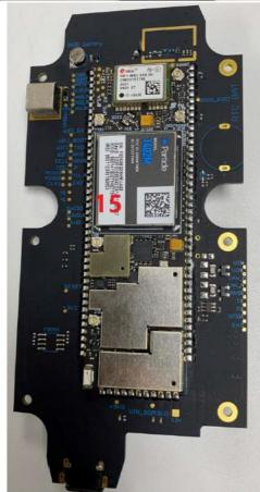
(Different models have different corresponding Cellular module models. Another model is T523M)
