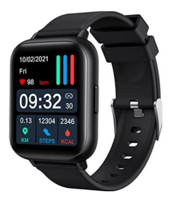
Press and hold the side power button to turn on the watch.
