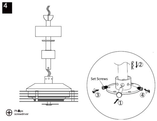
• Install the fan-motor assembly into the mounting bracket, taking care to install it in place.
