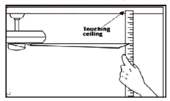
**WARNING:** TO REDUCE THE RI SK OF PERSONAL INJURY, DO NOT BEND THE BLADE ARM WHILE INSTALLING, BALANCING THE BLADES, OR CLEANING THE FAN. DO NOT INSERT FOREIGN OBJECTS BETWEEN ROTATING FAN BLADES.
