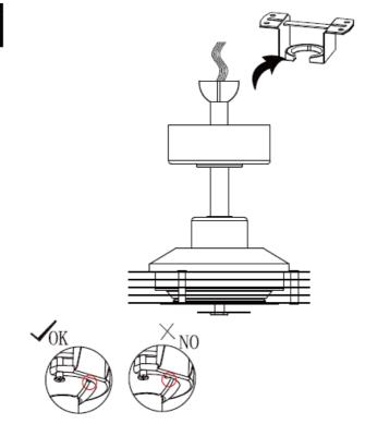
• Use the shoulder screw to lock the canopy to the mounting bracket.
