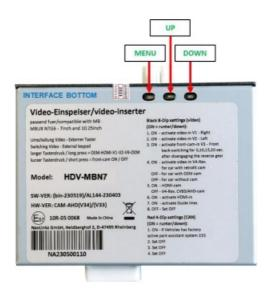
OSD menu settings can be changed using the 3 keypads on the back of the interface. MENU opens the OSD settings menu or moves the cursor to the next menu item. UP (UP) and DOWN (DOWN) change the values of the current menu item. The individual OSD settings menu of each video input can only be called up while it is displayed, regardless of whether a video source is connected. The following setting options are available in the OSD setting menus of the 5 video inputs:
