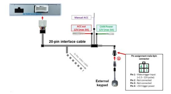
Connect the 4-pin female connector of the external keypad to the 4-pin male connector of the 20pin interface cable.
