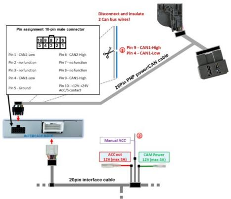
Disconnect and insulate the 2 CAN bus wires (grey, blue) of the 26pin PNP power/CAN cable approx. 4-5 cm behind the black male connector. Connect the violet wire Manual ACC of the 26pin PNP power/CAN cable to the +12V-+24V S contact (terminal 86s) or ACC terminal 15r (e.g. cigarette lighter, glove compartment lighting).
