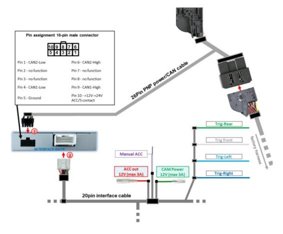
Connect the 10 pin female connector of the 26 pin PNP power/CAN cable to the 10 pin male connector of the interface. Connect the 20 pin female connector of the 20 pin interface cable to the 20 pin male connector of the interface.
