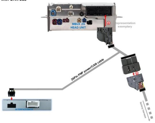
Disconnect the 26 pin female connectors of the vehicle wiring harness at the rear of the head unit and connect them to the 26 pin male connectors of the 26 pin PNP power/CAN cable. Connect the 26 pin female connectors of
