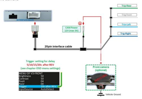
The green CAM Power 12V (max 3A) wire can be used to supply power to the front camera. This is only energised for the duration of the activation of one of the video inputs (some cameras are not suitable for continuous operation). Requirements for using the front camera is Dip 3 = ON (black 8 switch bench). The delay time can be selected in the OSD menu settings of the front camera for 5, 10, 15 or 20 seconds. Switching to front
