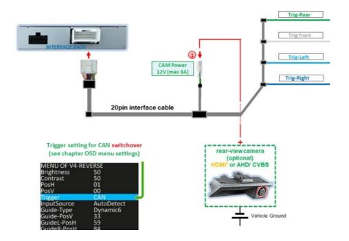
The +12V power supply for the after-market rear-view camera can be provided via the green wire CAM Power 12V (max 3A) of the 20pin interface cable, as voltage is only present on this wire when one of the video inputs is active (some cameras are not suitable for continuous operation).
