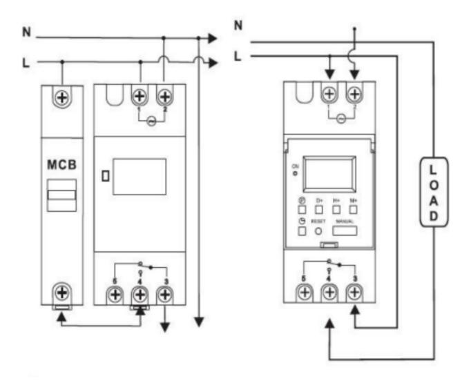
Connect the power source according to the input that is written on the side of the timer. For DC models use the connector 1 for the positive and connector 2 for the negative and for the AC models connect the Phase to connector 1 and connector 2 for the Neutral
