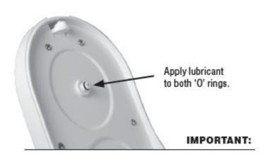
**NOTE:** The lid must be closed completely for the unit to function correctly with the internal fluid system. If the lid does not close completely or it sticks, then the two black 'O' rings on the underside of the cover may be dry and require a little lubrication. Apply a very thin layer of Vaseline to each 'O' ring with a Q-Tip. Just a thin layer is all that is necessary.
