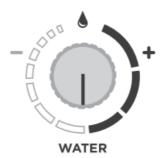
Observing the arrow printed on the control panel, turn the water control counter-clockwise to increase the flow, or clockwise to decrease water flow. If water does not flow through the insert when the foot pedal is depressed, the water passage in the scaling insert may be clogged.
