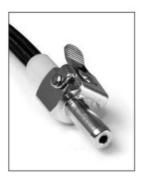
The male quick-connect that comes on the end of the water hose is the standard fitting presently used in the dental industry. If you are replacing a scaler that uses an Adec-type or other type of connection, remove the old fitting from the unit hose and attach it to the new water line. Check for leaks at all hose and filter connections before use, and tighten if necessary.
