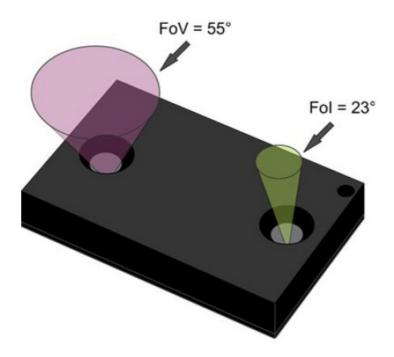
The emitter and receiver elements of the laser sensor form a cone shape. The emitter field of illumination (FoI) is 23°, and the receiver field of vision (FoV) is 55°. The LaserPING sensor will only sense objects within the FoI, but may have reduced sensitivity when bright objects are within the FoV. Readings may also be inaccurate when mirrored surfaces within the FoI scatter light to other objects within the FoI or FoV.
