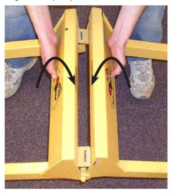
The support arms can be installed in a wide variety of positions depending on the support needs of the load being carried.
