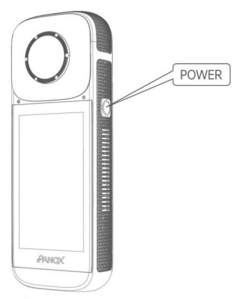
**Power On:** Press and hold the power button for 3 seconds.
