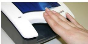
6. After replacing franking roller, connect device and perform franking on a test document. Sample franking will ensure the correct position and confirm proper installation of the roller.
