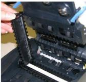
2. Remove any debris and dust. Clean the Contact Image Sensors with a soft, lint-free cloth dampened with Isopropyl Alcohol or with eye glass cleaner.
