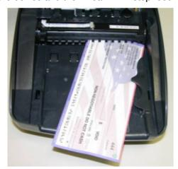
In this case remove and re-feed document into the scanner. Ensure that the top cover is properly closed after removing the document. If the device fails to recognize a document when inserted into the feeding tray, try opening the scanner to remove any paper or debris. Additionally, the feeding sensor and alignment sensors can be cleaned of any dust build-up with the use of canned air.
