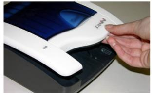
2. Open the franking cover by pressing forward on the top cover latches and pulling the franking cover down
