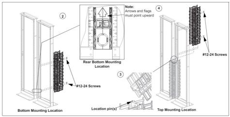
Installation Instructions R2PS using WMPVSMK side mounting kit
