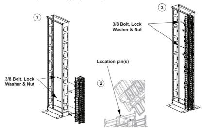
Installing Front Only Managers for Front and Back cable management.
