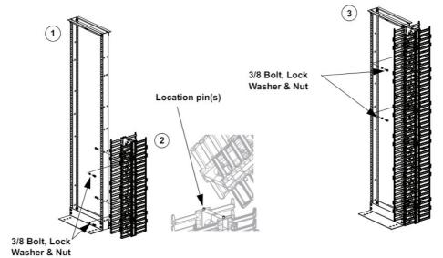
Installation Instructions Required mounting for R2P6S using WMPVSMK side mounting kit **Note:** Mount the racks to the floor (with the appropriate space between racks indicated in Table 2.)
