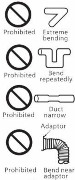
Do not install the unit where ducts are configured as shown in Fig A.
