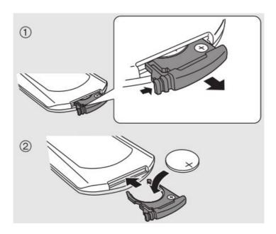
• Set the button-type battery with its (i) mark facing upward.
