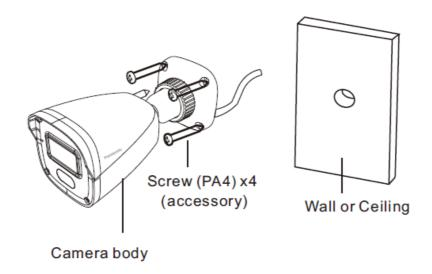
Step 1: Open a hole for cabling in the ceiling or wall.
