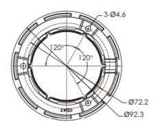
• Secure the camera with 3 screws (PA4) (accessory).
