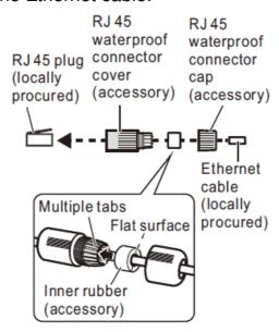
3. Insert the inner rubber into the far end of the waterproof connector cover (the direction in which multiple tabs are open) to secure it temporarily inside the multiple tabs.
